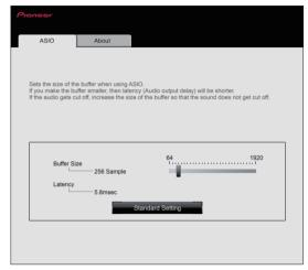
If the buffer size is made large, drops in audio data (breaks in the sound) occur less easily, but the time lag due to the delay in the transfer of the audio data (latency) increases.
