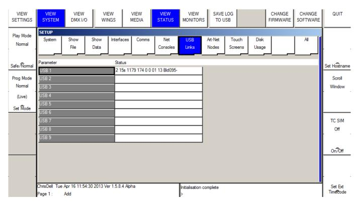
Put the cursor on the line for USB 1 as above. Press CHANGE FIRMWARE and select the new firmware file - e.g. CH331\_V1.0.hex. MagicQ should then say "Starting firmware upgrade" and then a few seconds later "Sent start upgrade".
