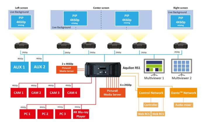
Aquilon RS1 can drive one 8K60p LED wall and 4x 4K60p AUX outputs
