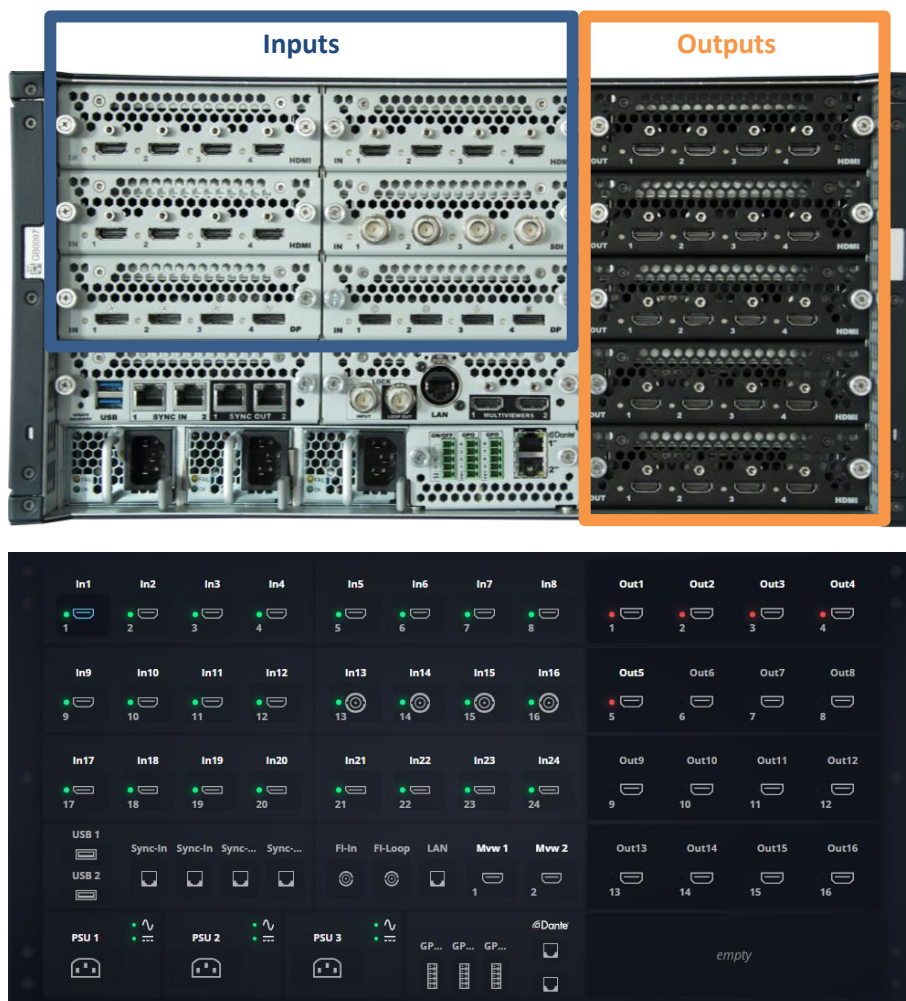
Fig. 2 - LivePremier rear panel (Aquilon C+) / virtual panel with Input/Output numbers (Aquilon RS4)
